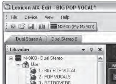
Double-click a program name to open it in the editor. The program settings are reflected in the Parameter knobs and buttons in the Program Editor window.
