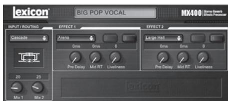
MX-Edit gives you all the same control and functionality as the MX400 front panel, with the exception of **Input** control and **System** functions.
