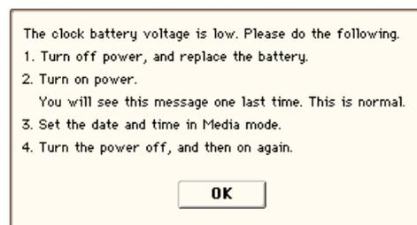
Make sure that you are not using a battery that has run down, and that the battery is installed correctly.
