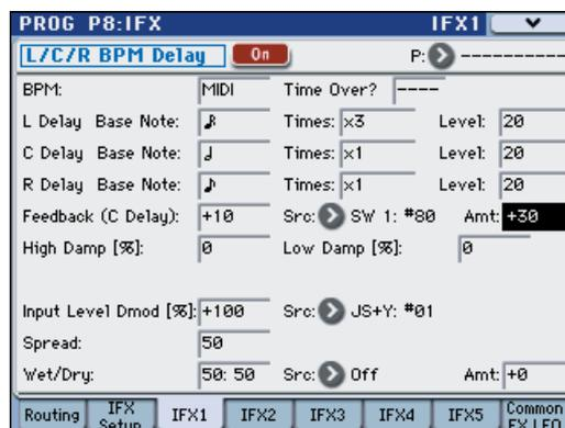
When you move the joystick away from yourself and press the SW1 switch, the feedback level will increase, and the delay sound will continue for a longer time. The Amt setting specifies the feedback level that will be in effect when the SW1 switch is pressed. If Amt is set to -10, pressing the SW1 switch will reduce the feedback level to 0.
