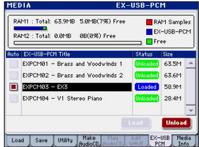
To load a different EX bank whose Status says "Unloaded" on a green background, select it by pressing its name and pressing the red Load box. Press OK when asked "Are you sure?" The Load process may take about 20 seconds.
